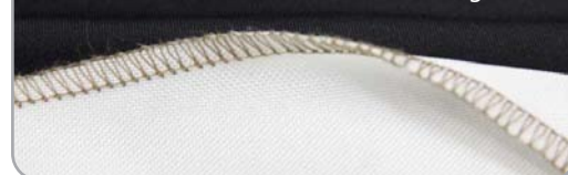
Flame Resistant Seam On Nomex Flight Suit
