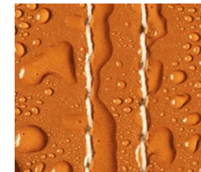
Water-repellent thread: No capillary effect
