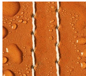
Thread without water-repellent finish: Capillary effect
