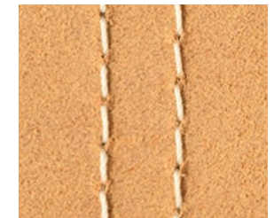
Water-repellent thread: No water absorption
